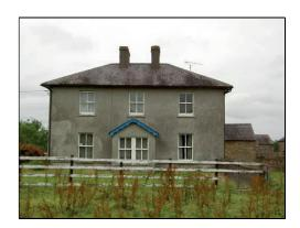
Hipped roofs can be utilised to reduce the visual bulk of square plan houses, an effect that is negated where chimneys are placed at either gable end.
