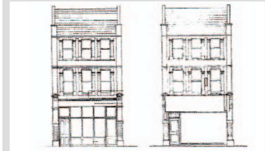
Examples of good and bad shop front design – shop front should relate to the upper floors, particularly with respect to glazing. Separate access to upper floors should be maintained.
