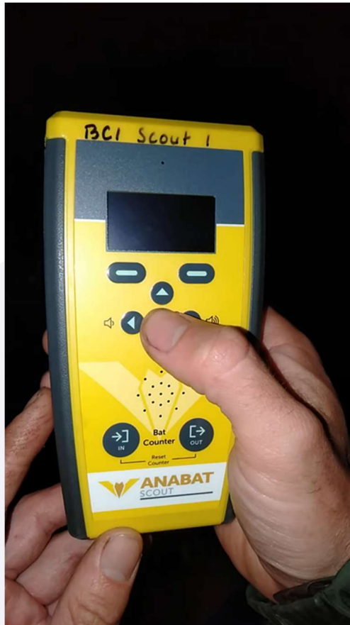
Figure 4. The Anabat Scout full spectrum bat detector used for the surveys.
