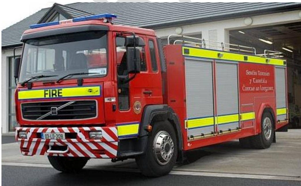
Photo 11 Longford town fire engine with a polycarbonate body
