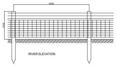
3 ROWS GALVANISED BULL WIRE FIXED TO 150MM DIA. TREATED OCTOPOSTS WITH 38MM
