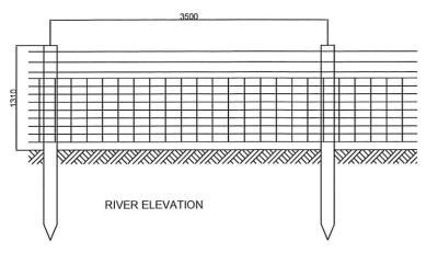
3 ROWS GALVANISED BULL WIRE FIXED TO 150MM DIA. TREATED OCTOPOSTS WITH 38MM STAPLES.
