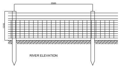
3 ROWS GALVANISED BULL WIRE FIXED TO 150MM DIA. TREATED OCTOPOSTS WITH 38MM STAPLES.
