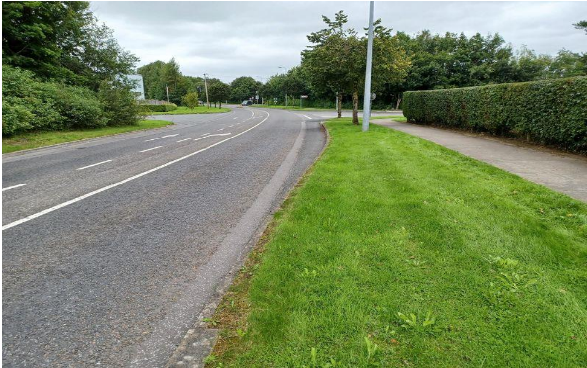
View continuing along N63 from town centre to N4 Roundabout showing existing path, hedge and Public Lighting columns. It is proposed to reinstate the old kerbline when Junction Tightening.
