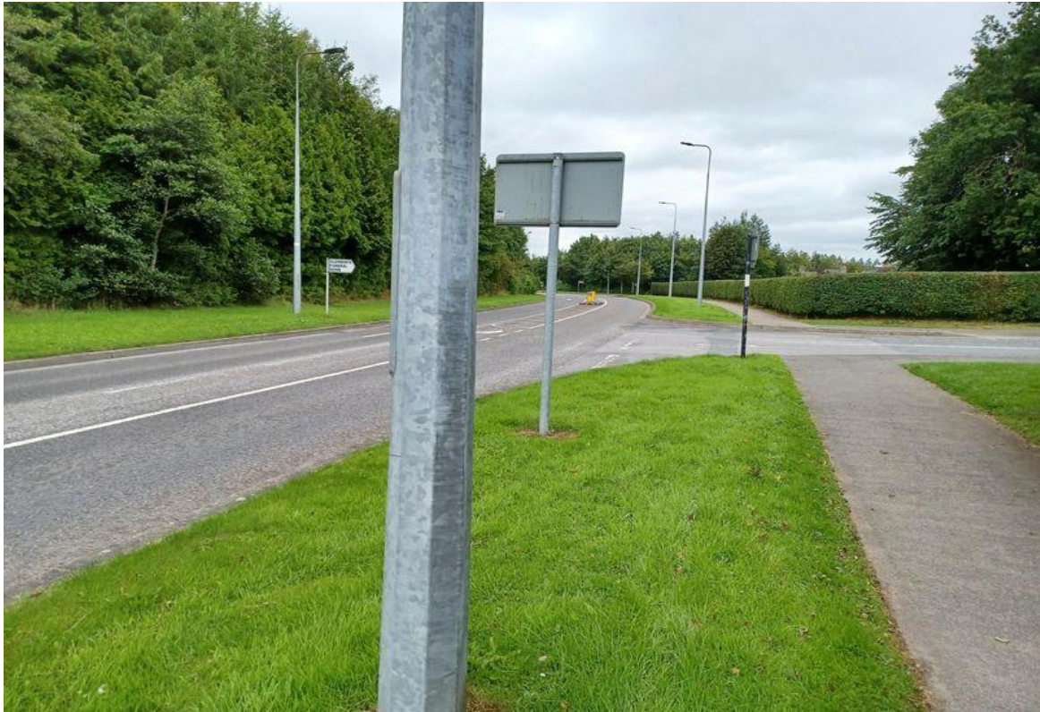
View continuing towards junction for Oaklands Estate and traffic exit from St. Eimears N.S. It is proposed to move all Public Lighting Columns in this photo to the rear of Existing footpath.
