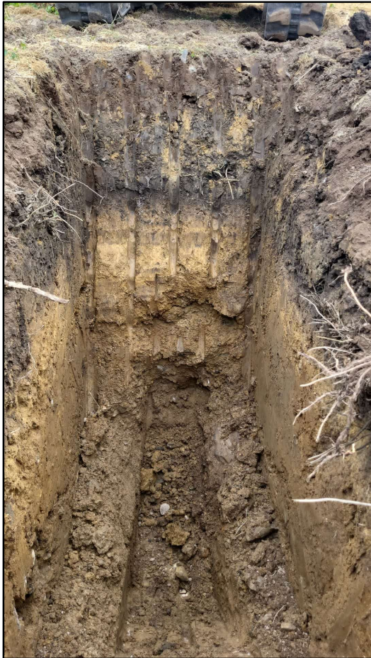
Fig. 2 & 3. (Above) A trial pit depth of >2.5m was achieved with no evidence of groundwater at depth.
