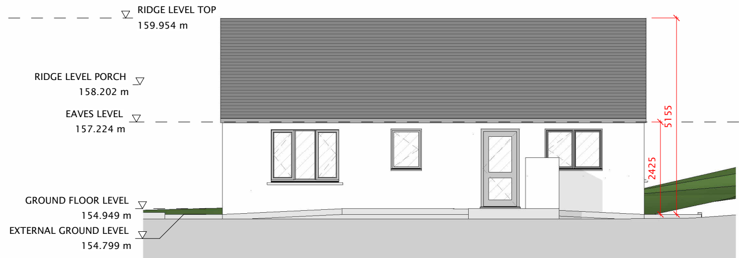
1 EAST ELEVATION - Design 1 : 100
