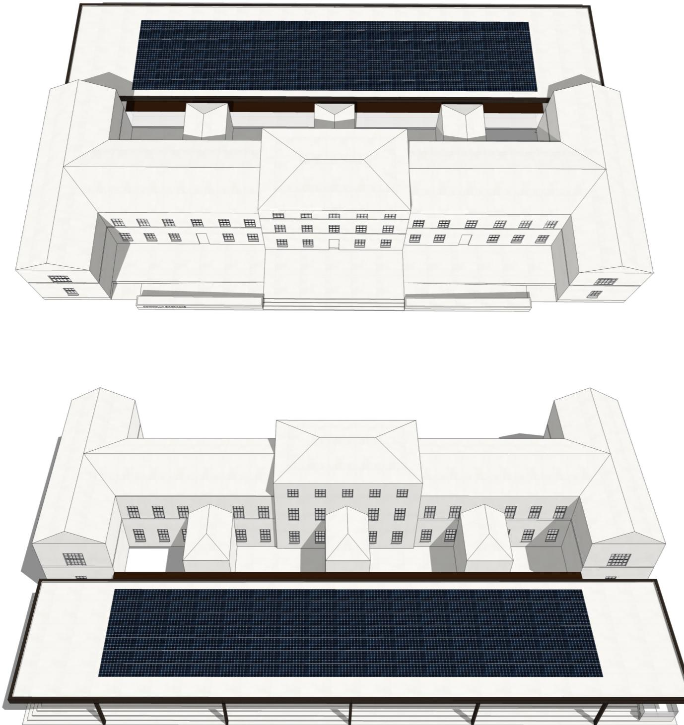
3D aerial view from east and west showing relationship of proposed extension to existing building. Note solar photovoltaic panels provided on roof of extension for passive energy generation strategy.
