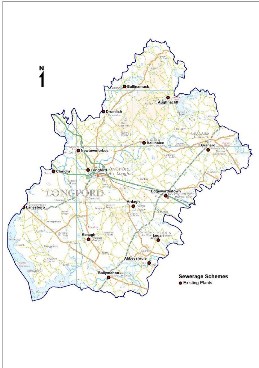
Figure 5.2: Sewerage Schemes in County Longford
